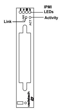
FIGURE 2. AMC302 Front Panel
