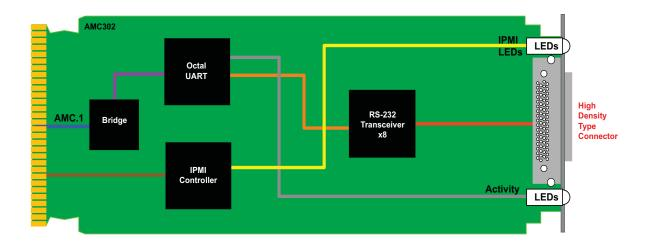
FIGURE 1. AMC302 Functional Block Diagram
